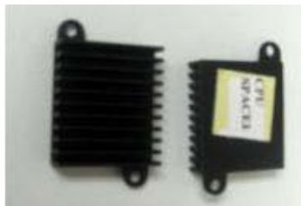
CPU Spacers (2) (to increase air circulation)
